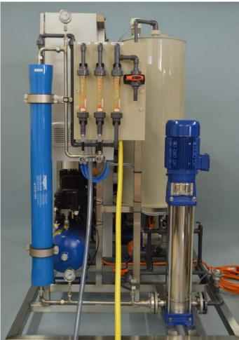
The reverse osmosis unit sterilizes the water by removing all remaining impurities. The reverse osmosis unit features two outlets: one for the cleaned, treated water (permeate) and one for the concentrate, water which contains relatively more soluble substances than the permeate.
